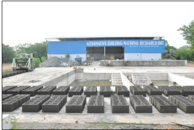
Alternative Building material research unit - Building materials like hollow blocks, interlocking blocks and paver blocks are manufactured.
