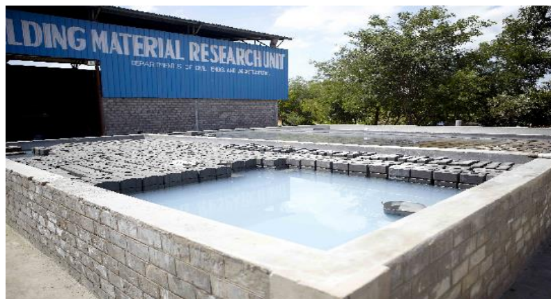
Alternative Building material research unit - Building materials like hollow blocks, interlocking blocks and paver blocks are manufactured.
